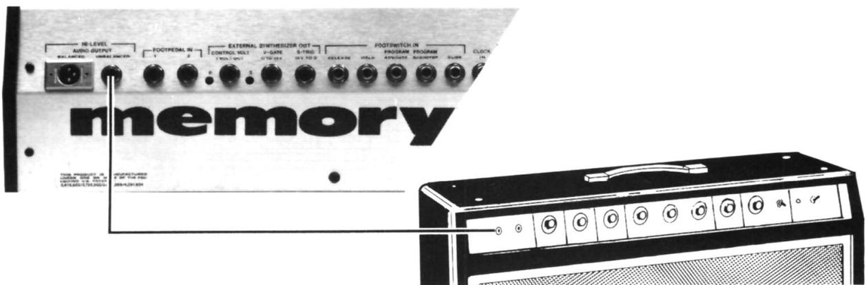
Turn the output volume of both the Memorymoog and the amp down to zero. Turn the Memorymoog on and then turn the amp on. Bring the volume of the amp up to where you're used to setting it. While holding down a note, bring the MASTER VOLUME control (at the upper right corner) up until it's at a comfortable level.
